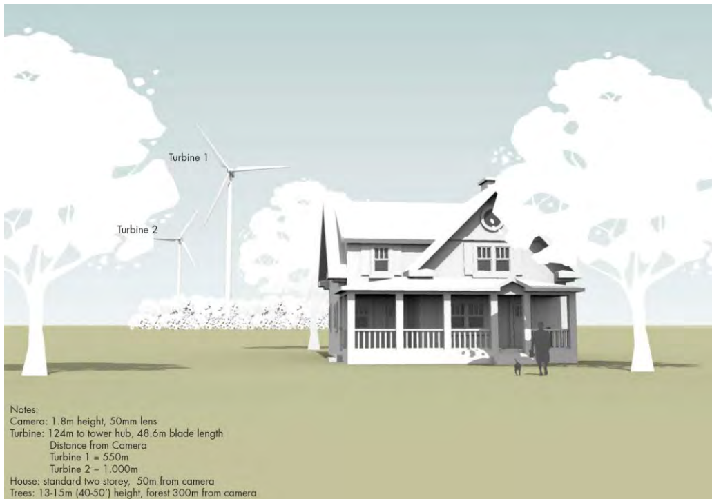
Visual Aid 2: Wind Turbine Scale Schematic, with trees (124m hub height)
